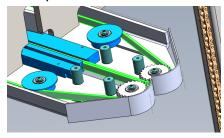
The bag top travels between two forced air heat manifolds followed by compression rollers, giving an approx seal of 1⁄4 inch at the top of the bag.
